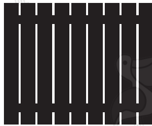
STEPNEY 65x16 Battens Top View Minimum Gap 20mm
